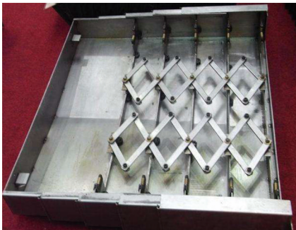
图1 引兴公司的铰链式导轨防护罩 Fig.1 Hinged guide rail protective cover of Yinxing company
